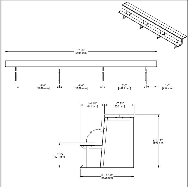
SEATS ARE CONSTRUCTED OF 10" [254 mm] WIDE ANODIZED ALUMINUM. FRAMEWORK IS COMPRISED OF WELDED HEAVY GAUGE ALUMINUM ANGLE FOR SUPERIOR SUPPORT AND STRENGTH. END CAPS ARE CONSTRUCTED OF DIE CUT ALUMINUM STRIPS WITH PUNCHED HOLES FOR SCREWS OR RIVETS.
