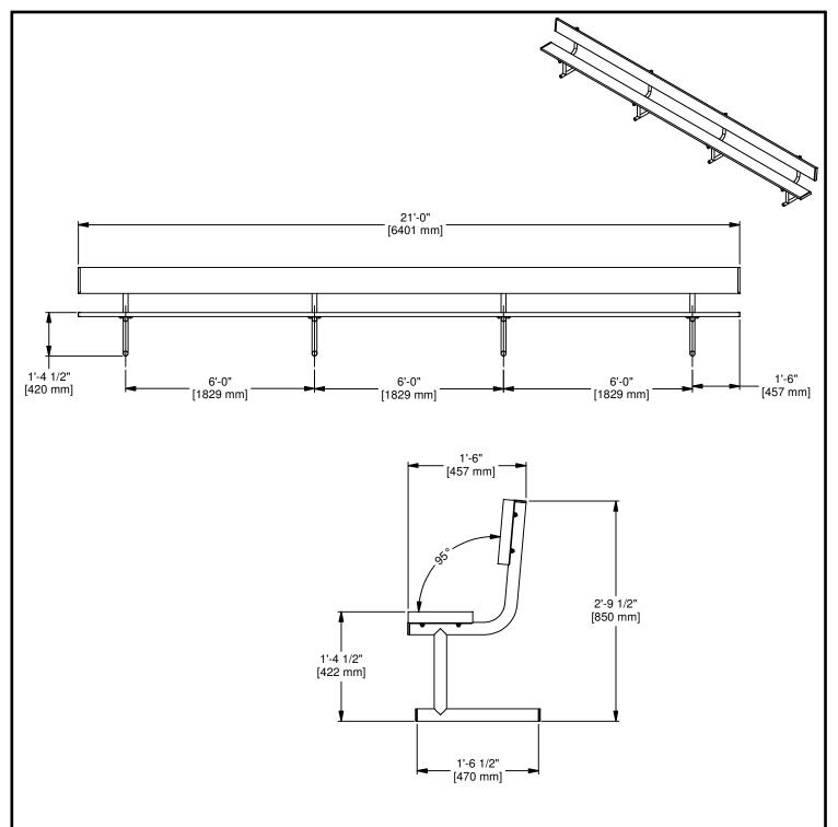
SEATS ARE CONSTRUCTED OF 10" [254 mm] WIDE ANODIZED ALUMINUM. FRAMEWORK IS COMPRISED OF WELDED HEAVY GAUGE STEEL TUBING FOR SUPERIOR SUPPORT AND STRENGTH. END CAPS ARE CONSTRUCTED OF DIE CUT ALUMINUM STRIPS WITH PUNCHED HOLES FOR SCREWS OR RIVETS.
