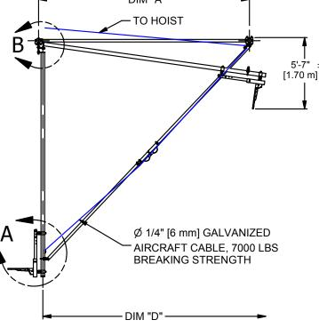
NOTE: DIM "C" IS 63" [1600 mm] WITH A RECTANGULAR BACKBOARD AND 35" [889 mm] WITH A FAN SHAPED BACKBOARD
