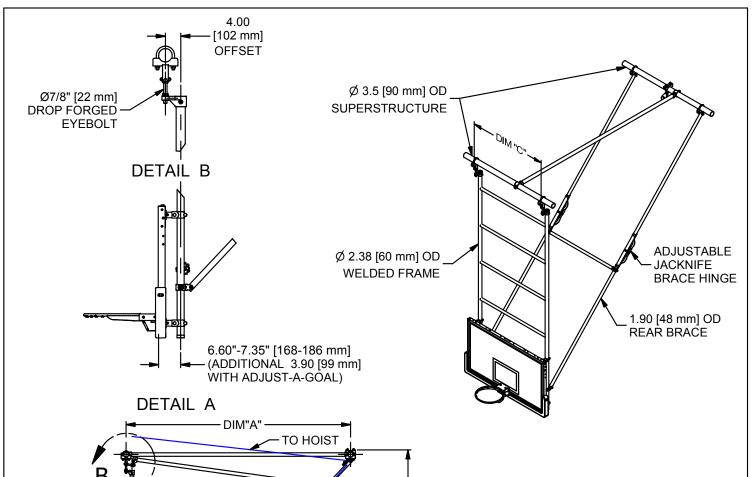
NOTE: DIM "C" IS 63" [1600 mm] WITH A RECTANGULAR BACKBOARD AND 35" [889 mm] WITH A FAN SHAPED BACKBOARD
